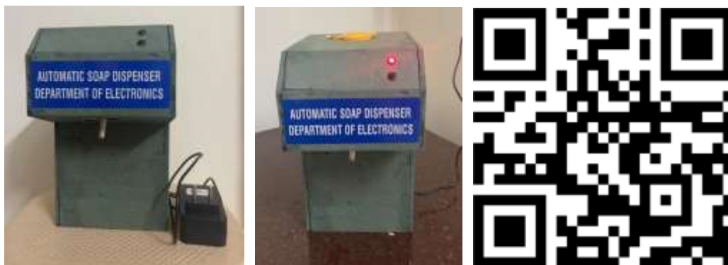
Figure 5: Working Model of developed Automatic Liquid Soap Dispenser with QR code
